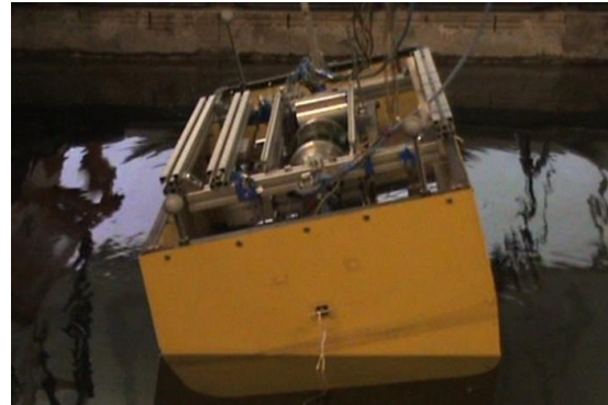
Figure 1 Cylindrical section of a RO-PAX vessel subjected to forced roll in calm water.
