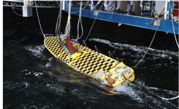
Fig. 2: High roll motion without capsize and very low amount of green water in stern quartering seas.
