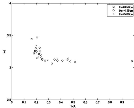
Fig. 1: Kurtosis plotted against directional spreading ( $1/A$ ) where  $A$  is defined as  $A \cdot K(\theta; f) \equiv G(\theta; f)$ , and  $G(\theta; f)$  is the directional distribution function satisfying  $\max_{\theta} K(\theta; f) = 1$ ; circle 35-40 m, square 14-15 m fetch. The figure is reproduced from Waseda et al. (2009a).
