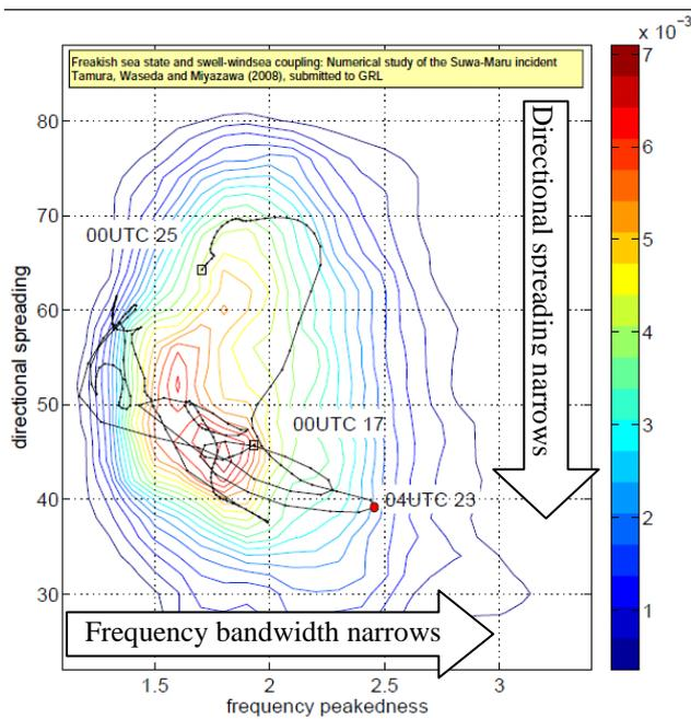
Fig. 2: The trajectory of spectral property in the  $Q_p - \sigma_\theta$  diagram. The occurrence of freak wave is highest in the lower right corner and lowest in the upper left corner. The figure is reproduced from Tamura et al. (2008). Case 1 in this paper.
