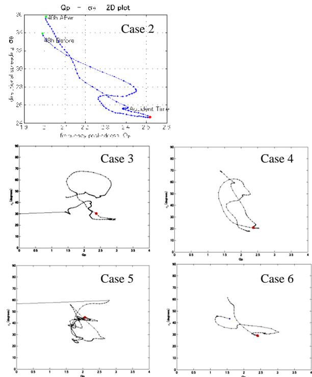
Fig. 3: The trajectory of the spectral property in the  $Q_p - \sigma_\theta$  diagram for cases 2 to 6. Except for the fifth case, the accident occur (red dot) at the lower right corner of the diagram when the directional spectrum is narrow.
