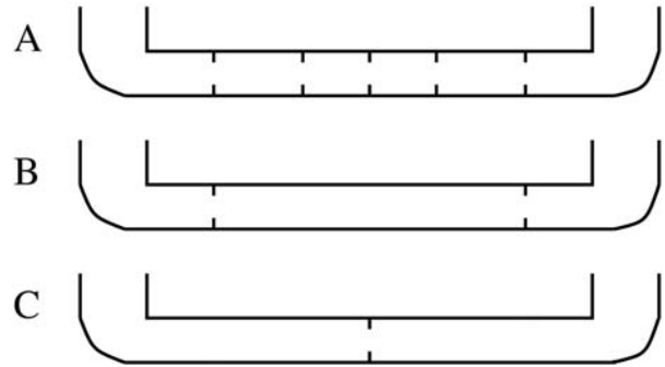
Fig. 2: Schematic representation of the different detail levels for modelling of the cross-duct
